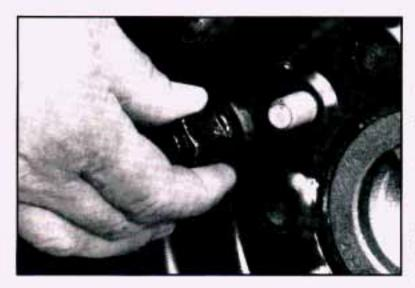
Put on the spare tire. Put the nuts on by hand. Make sure the cone-shaped end is toward the wheel. Tighten each nut by hand until the wheel is held against the hub. If a nut can't be turned by hand, use the extension and see your dealer as soon as possible.
